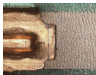
Extended focus image (EFI) of a crimped terminal
